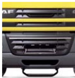
New steps with three rungs for further reduction in susceptibility to damage. The middle rung is fixed to the chassis and the flexible bottom rung is suspended.
