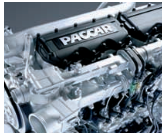
DAF EEV engines are based on the new Euro 5 engines and fitted with a passive soot filter.
